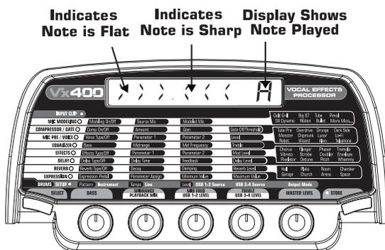
In Tuner mode, you can change your tuning reference. The default factory setting is A=440 Hz. (displayed as A=440). Rotate the Number 1 Knob to select alternate dropped tunings. Alternate tunings are A = Ab , A = G , and A = Gb. The display window briefly flashes the selected tuning preference.
