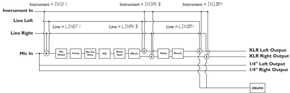
**1/4 MOD** - The Mic signal with the Modulation Effects is routed out the 1/4" outputs only. All other sources and Mic with all Effects are routed out the XLR outputs.
