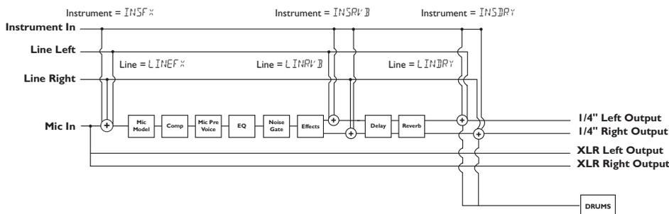
**XLRMOD** - The Mic signal with Modulation Effects is routed out the XLR outputs only. All other sources and Mic with all Effects are routed out the 1/4" outputs.
