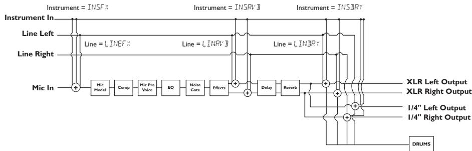
**XLRDRY** - The dry Mic signal is routed out the XLR outputs only. All other sources and Mic with all Effects are routed out the 1/4" outputs.
